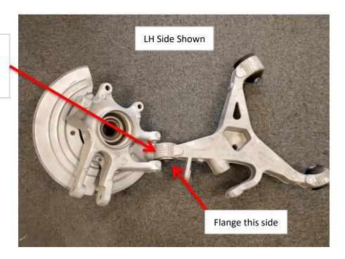
x2 1L washers to be fitted either side of 31BF Polybush to both sides of the vehicle where there is 59mm gap between the brackets.
