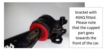
When the bracket is fitted back to the car the cupped end must face forward.
