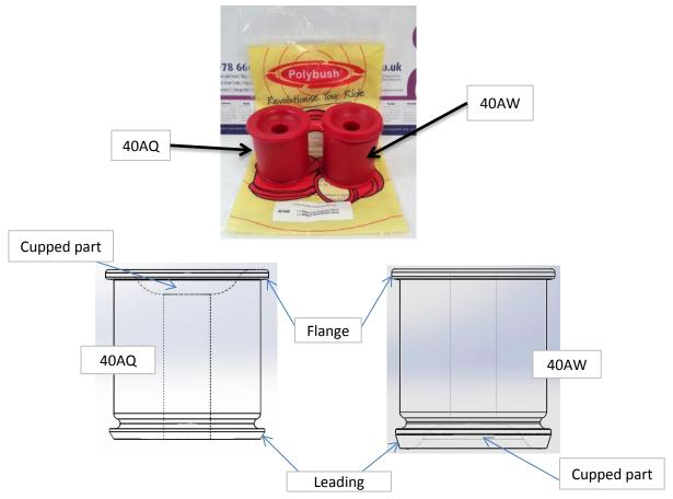
The brackets on your model are not handed: one end of the bracket has a turned in lip, this lip will face towards the front of the vehicle on one side and towards the rear on the other side. Note that the cupped end of the bush must always face forwards towards the wishbone.
