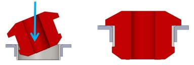
Step 5 Insert tube until flush.
