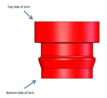
No grease is required. Use tyre soap or washing up liquid to aid with fitment.
