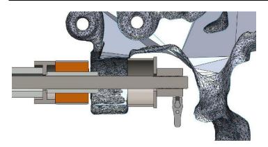
Step 4: Wind in bush until flush with either side of the housing eye for 27AL & 27AR. Note: Ensure 27AQ & 27AP flanges are fully seated. (I.e. Both flanges should be fully visible).
