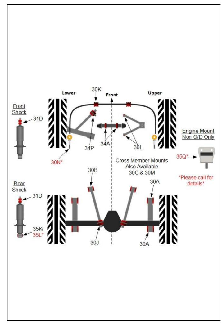
Vehicle suspension geometry must be checked / reset once bushes have been fitted. ALL Part Kits Are Available Separately. O.E.part numbers for reference only This Price list is subject to our standard conditions of sale, a copy of which is available on request and is exclusive of VAT & carriage. E & O E.
