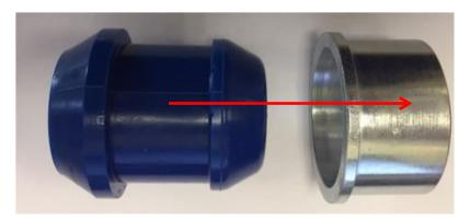
With the sleeve inserted into the arm, now press the polyurethane bush into the sleeve – Note the direction of insertion (small diameter into flanged end of sleeve). Washing up liquid should be used to ease the insertion process.
