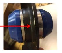
Following the removal of the OE bush press the steel sleeve into the bore of the arm – Note the direction of insertion (sleeve flange against raised bore of the arm)
