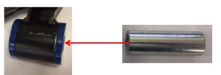
Following the removal of the OE bush push both halves of the polyurethane top hat bushes into the housing from each side.
